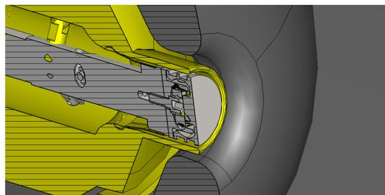
Figure 3: Sectional view of the puck inside the stalk.
