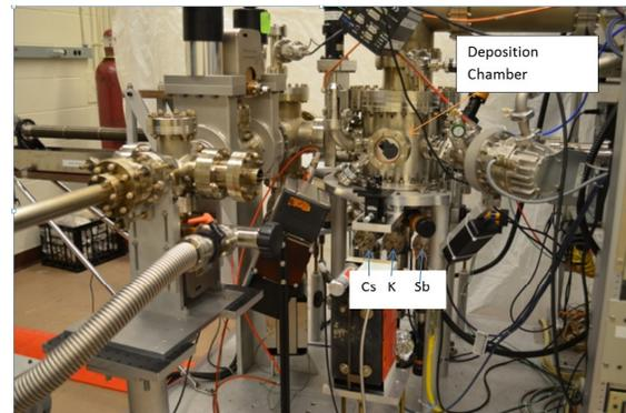
Figure 5: Multi-alkali deposition system for the 112 MHz gun.
