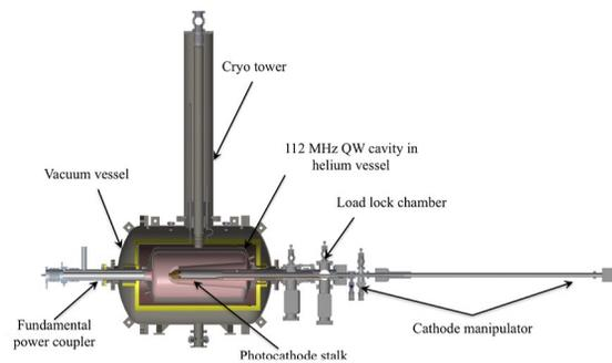
Figure 1: Cross section of the 112 MHz SRF gun (elevation view). The laser light is entering the gun through a hollow fundamental power coupler, which also provides an exit path for the electron beam.
