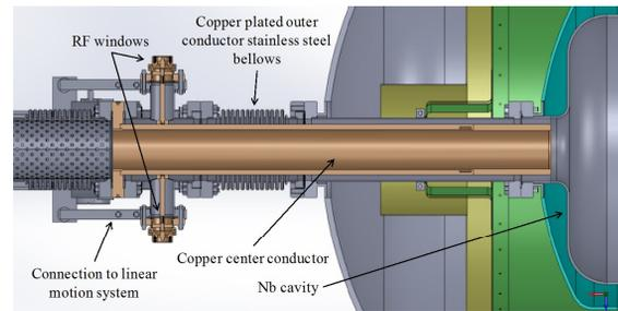
Figure 4: Cross section of the FPC attached to the beam-exit port.
