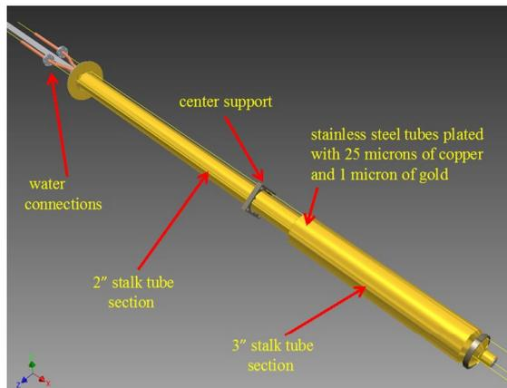
Figure 2: Cathode stalk assembly.
